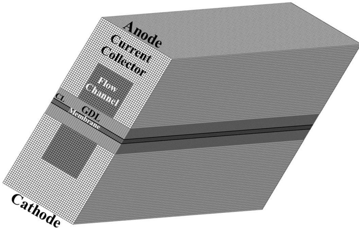
Figure 1: Grid structure of PEMFC model
