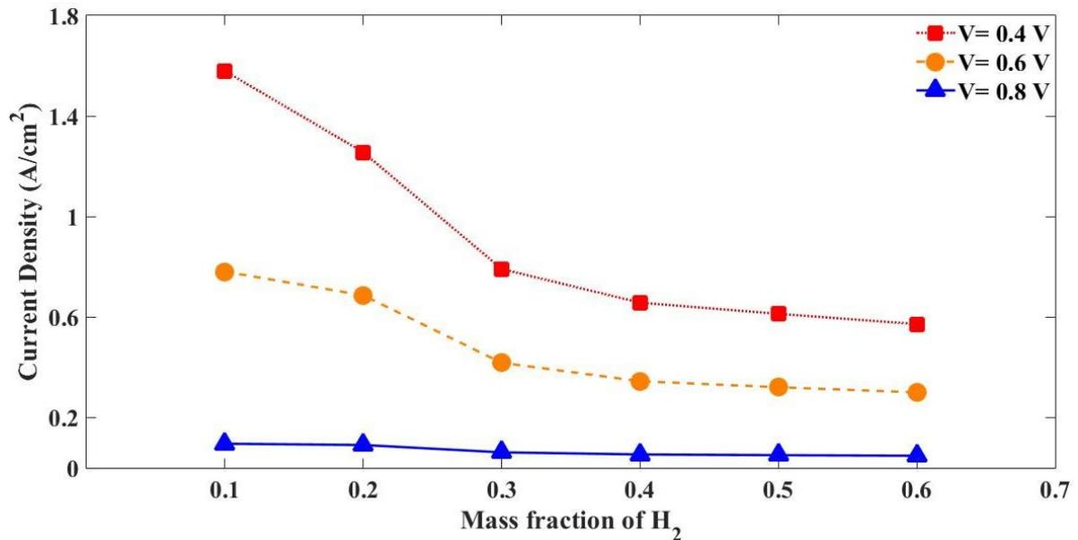
Figure 3: Change of current density for different mass fractions of hydrogen at various cell voltages of 0.4-0.8 V
