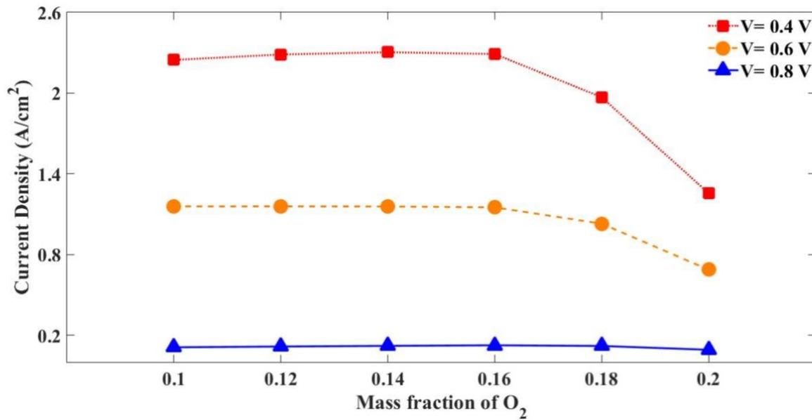
Figure 4: Change of current density for different mass fractions of oxygen at various cell voltages of 0.4-0.8 V
