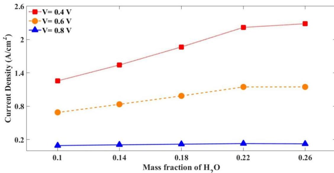
Figure 5: Change of current density for different mass fractions of water (cathode) at various cell voltages of 0.4-0.8 V
