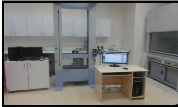
Figure 9: Universal tensile test machine
